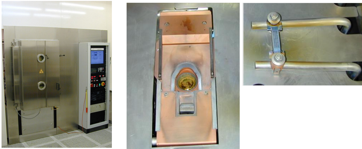
Figure 4. Left: Lab600 evaporator. Middle: e-beam evaporation source. The material is placed in the circular crucible in the middle and heated using an electron beam. Right: boat for evaporation via Joule heating.
